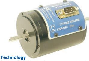
An extensively developed measurement principle is used, in which the intensity of light beams is measured by means of photovoltaic detectors, and the electrical output is used to provide precise indication of the applied torque transmitted by the shaft.
