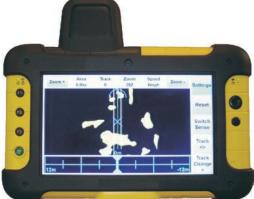
The <u>HELINAV TRACKMASTER</u> system is also compatible with the <u>HELINAV LOADMASTER</u> load sensor, when used together it allows lifted weight and drops to be recorded to file for future billing purposes.
