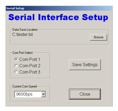
The Serial Interface Setup window allows configuration of the negotiation speed with the RS232 interface in the readout, as well as what port to use.
