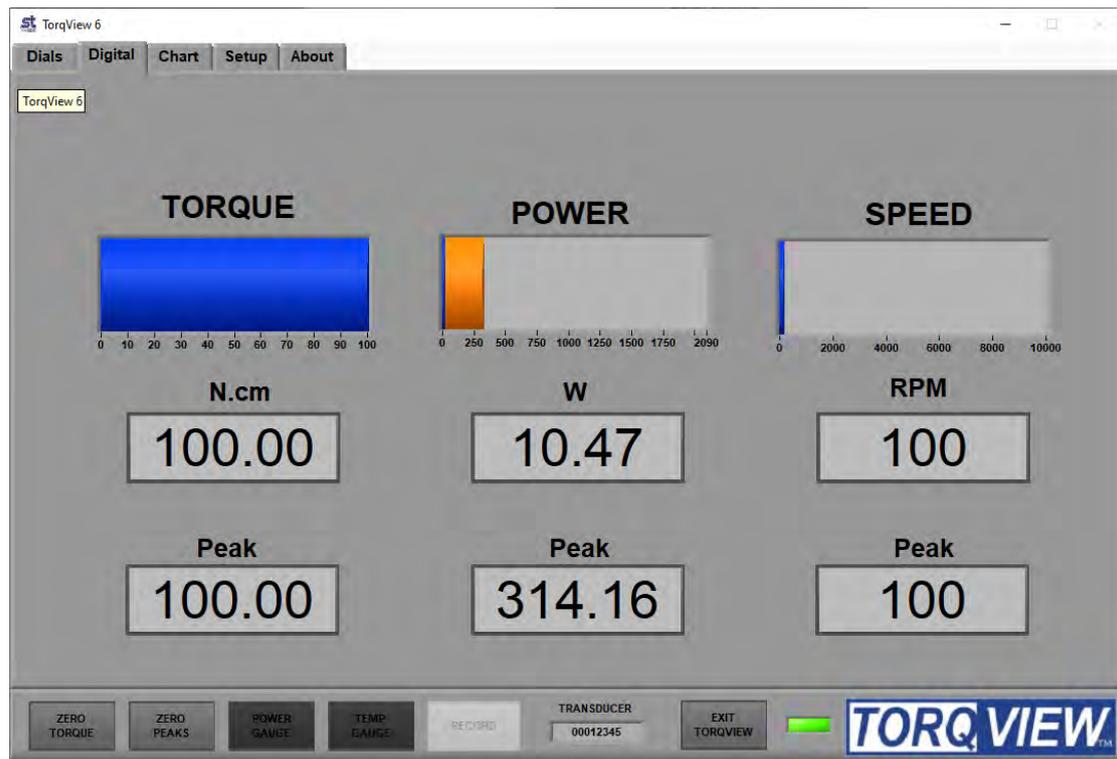
The Digital Screen displays the same data, less temperature, as the Dials Screen but as digital bars. The blue coloured bar displays the actual data, whereas the orange coloured bar, as an underlay of the blue coloured bar, displays peak value. Actual and Peak values are also displayed as numeric values under the coloured display bars.
