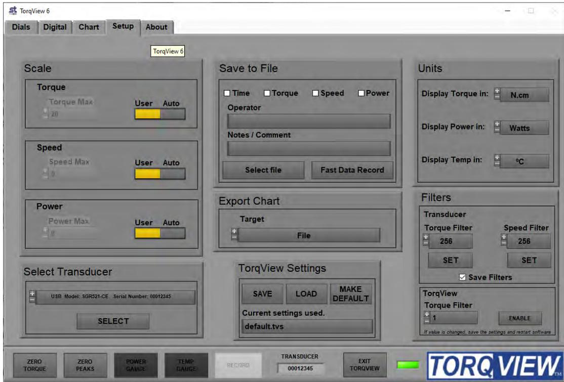
The Setup Screen is used to select the scales and units displayed on other screens as well as to select other options.
