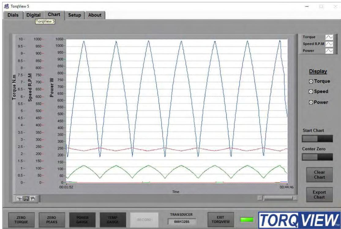
The Chart Screen displays the data onto a chart. Scales are automatically set at initialisation or user set via the Setup Screen.
