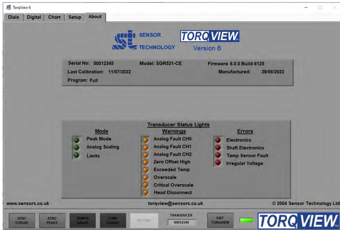
The About Screen displays the TorqView version and whether it is a Demo or Full program. The Demo program will display how many minutes remain. Both programs will also display the Serial No. of the active transducer, the date of its last calibration, its manufactured date the firmware version and the Transducer Status Lights diagnostic box.
