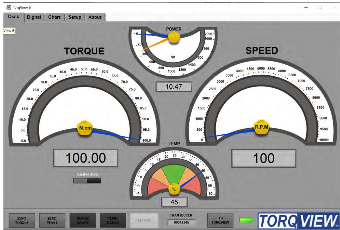
The Dials Screen is the main TorqView screen and displays torque, speed, power and temperature.
