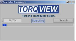
A 'Searching' text will flash blue and an indicator will show the progress. This may take a few minutes depending on the number of ports. When the transducer connected to its port has been found, it will be displayed in a drop down menu. If more than one transducer has been found it will display all of them in a drop down menu. Select which transducer to use.
