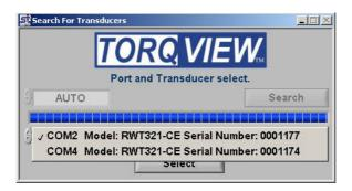
The selected transducer will now be connected and the 'Search For Transducers' screen will disappear and be replaced by the Dials Screen.
