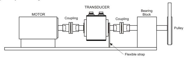
When using a pulley or pulleys it is recommended a bearing block or blocks should be used to ensure bending loads are not transmitted to the transducer. Care should be taken not to induce any end loads or bending moments to the shaft, as these may induce inaccuracies to the torque measurement and in extreme cases damage the transducer.
